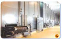
Fully welded stainless steel wall panel enclosure
