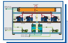
The multi-compressor Brine Chiller satisfies all the needs for secondary refrigerant application in the negative range of temperature.
